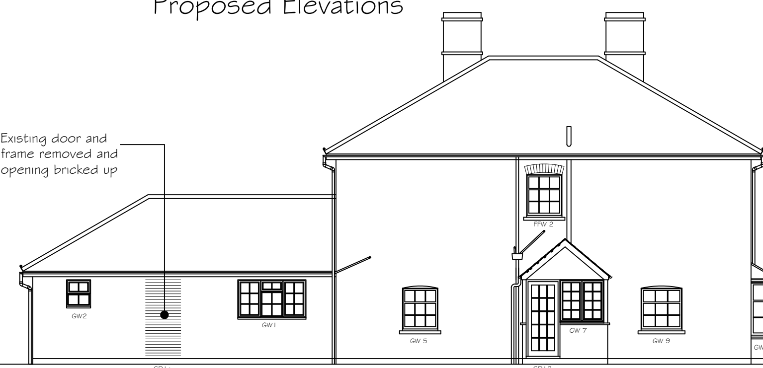
Front Elevation [ North East ]
