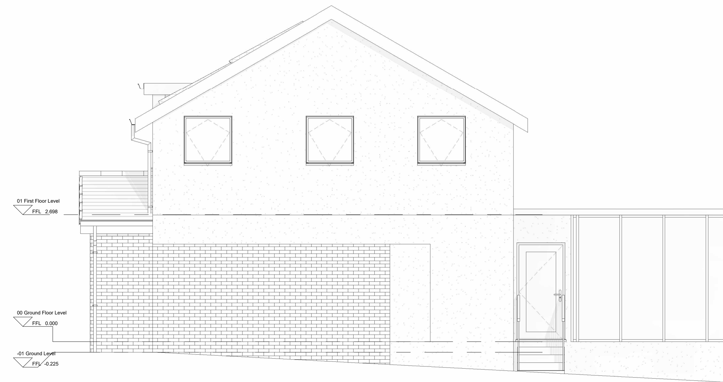
Gable Elevation - Proposed 1 : 50
