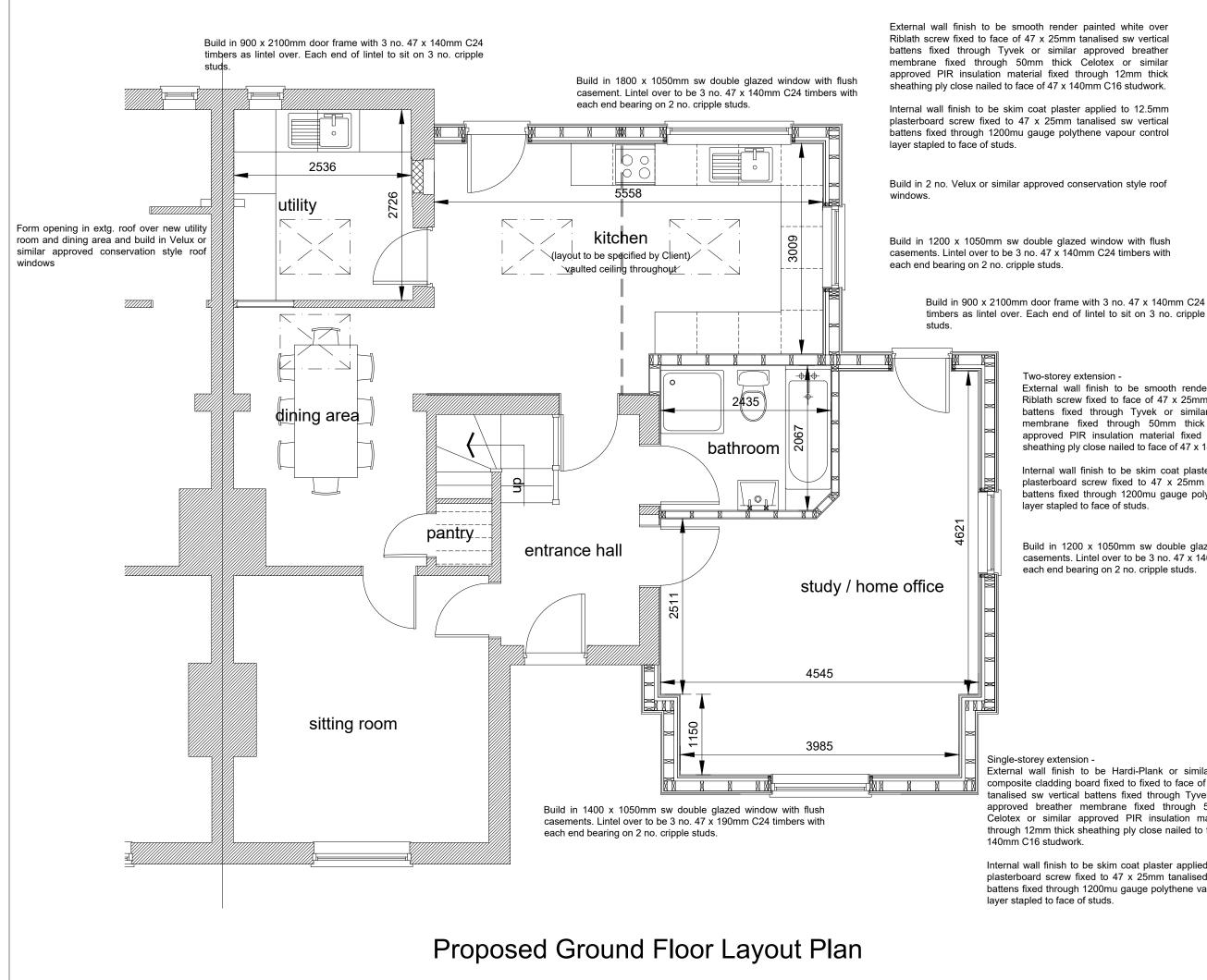
External wall finish to be smooth render painted white over Riblath screw fixed to face of 47 x 25mm tanalised sw vertical battens fixed through Tyvek or similar approved breather membrane fixed through 50mm thick Celotex or similar approved PIR insulation material fixed through 12mm thick sheathing ply close nailed to face of 47 x 140mm C16 studwork.
