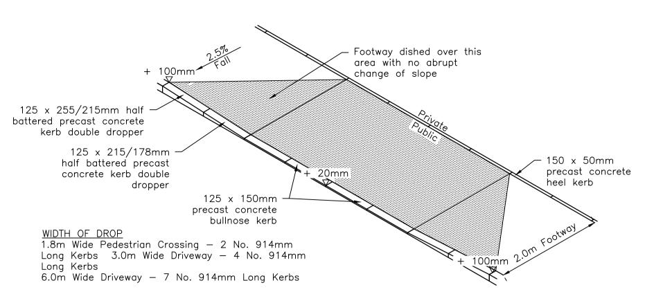
TYPICAL VEHICLE CROSSING DETAILS 100mm KERB UPSTAND
