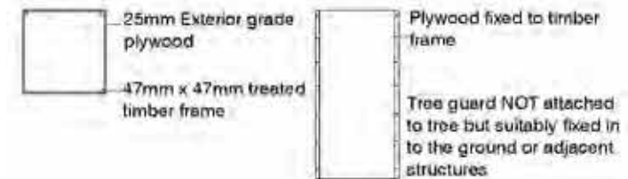
Fig 3 - Temporary Protective Fencing.
