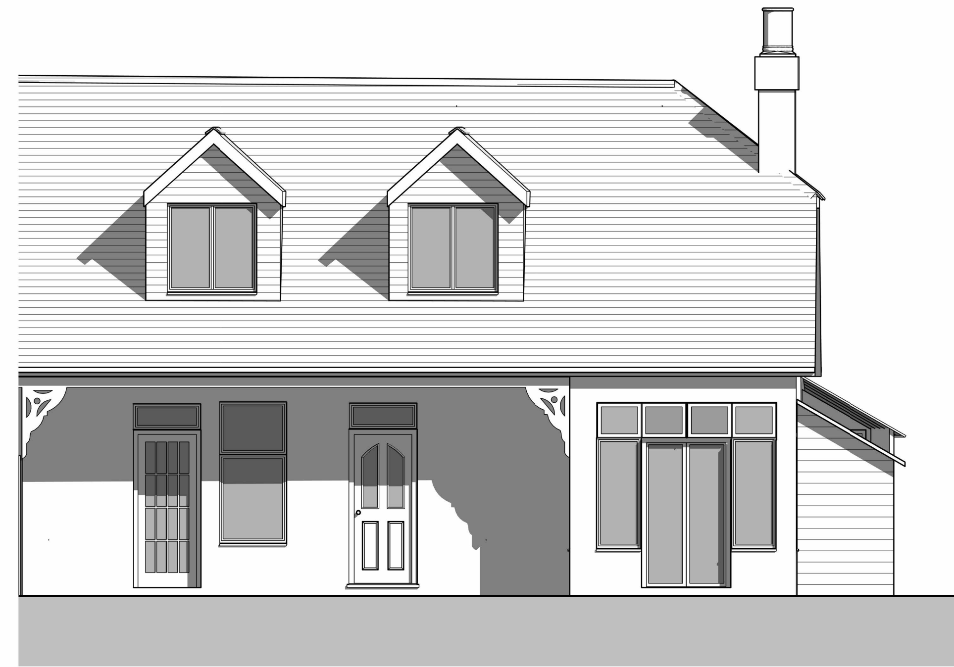
2 Proposed South East Elevation 1 : 50
