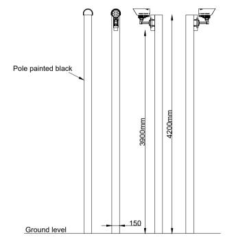
NOTE: Dimensions and drawings of cameras taken from MAV systems Ltd.
