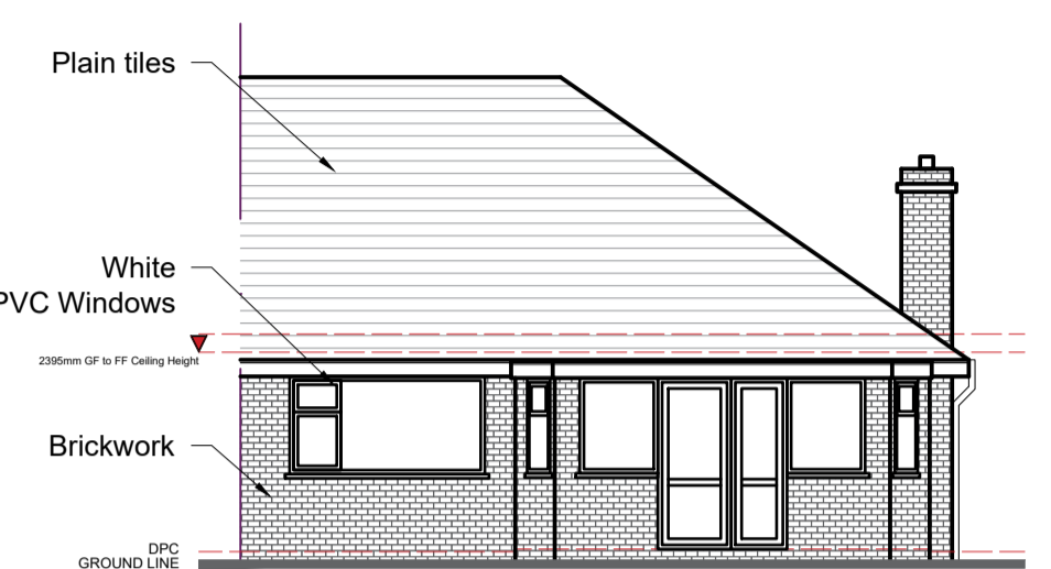
Existing South West Elevation Scale: 1:100
