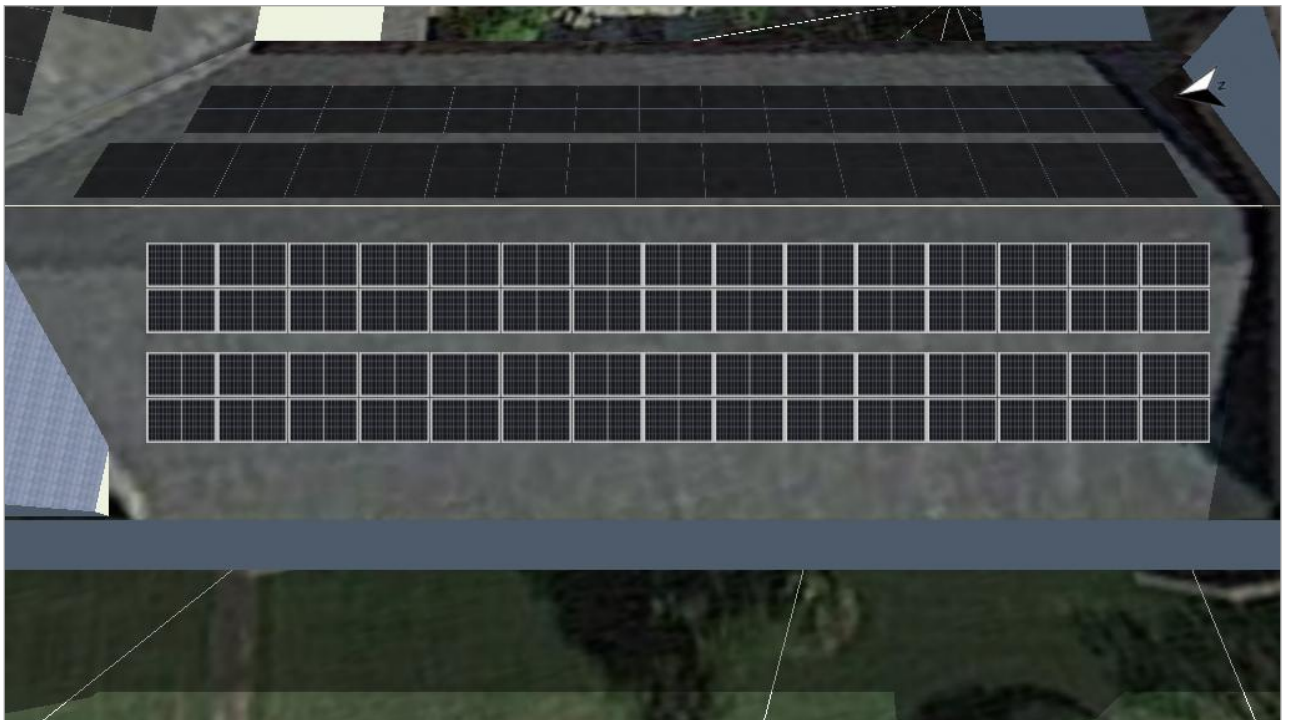
Figure: 4. Module Area - Building 03-Roof Area West
