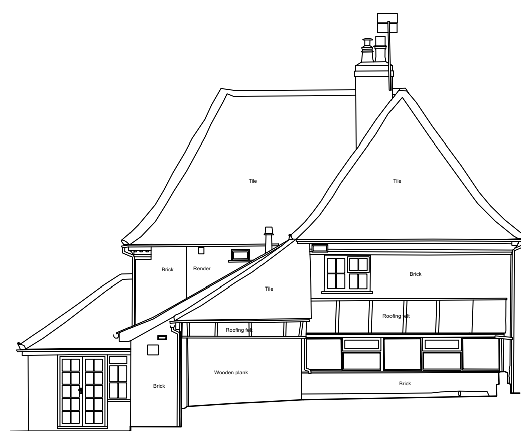
B ELEVATION B: Farmhouse South Elevation as Existing 1:100
