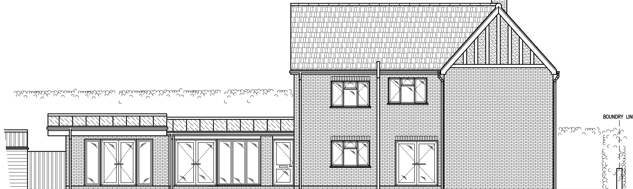
EXISTING SIDE ELEVATION (1:100)
