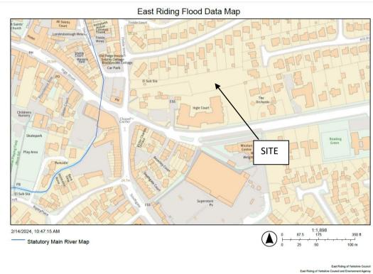
Weighton Beck (main river) is culverted to the west of the site and may provide an outfall for surface water from the development.
