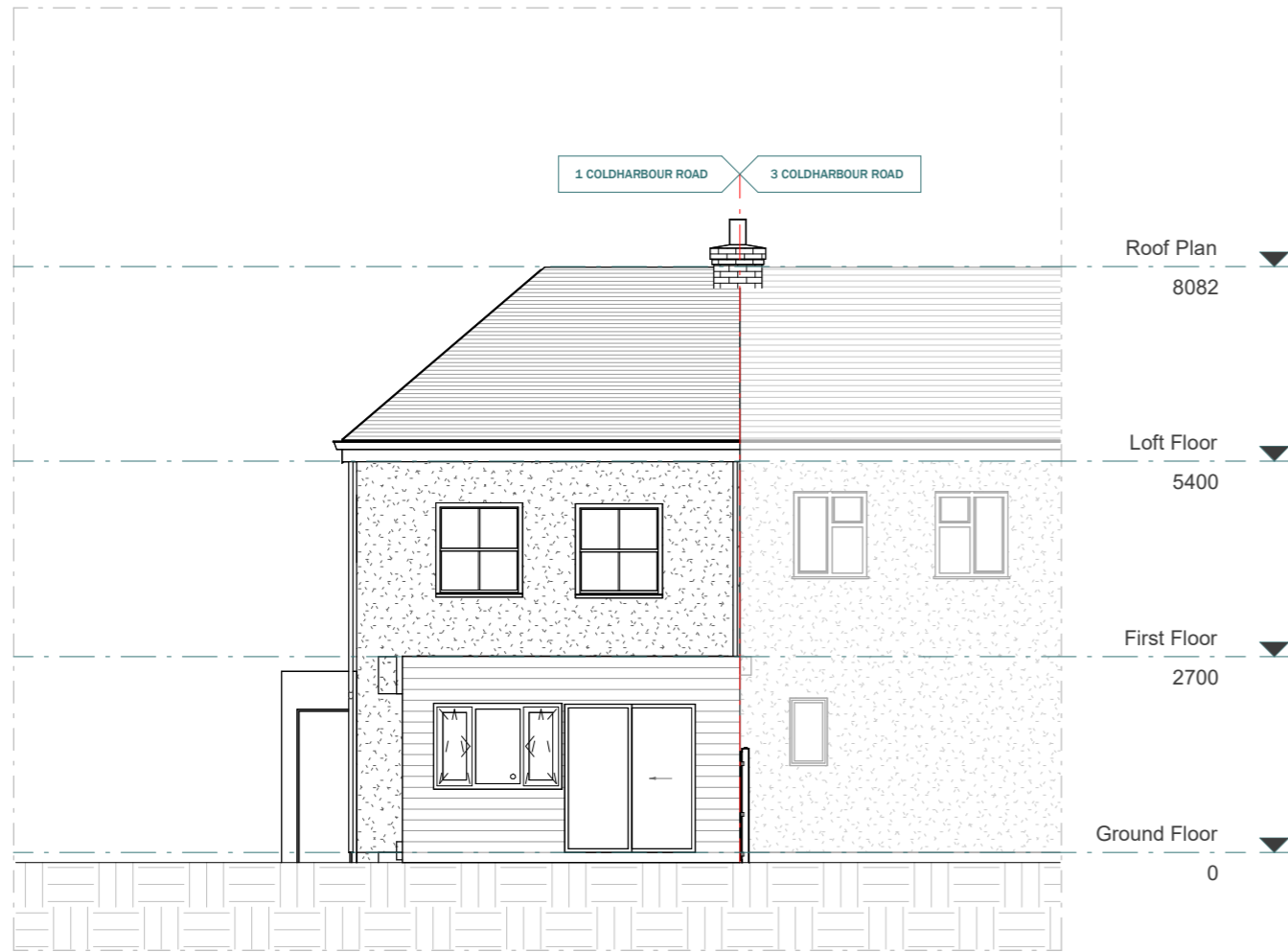
EXISTING REAR ELEVATION
