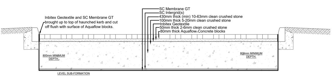
TYPICAL SECTION THROUGH FORMPAVE AQUAFLOW ATTENUATION SYSTEM
