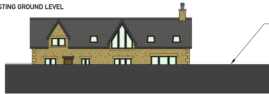
PROPOSED REAR ELEVATION SHOWING EXISTING GROUND LEVEL
