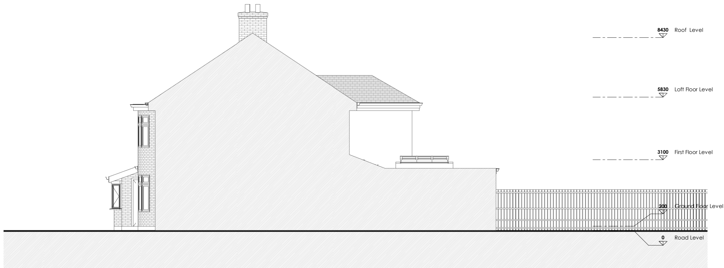
Proposed Side Elevation 1 ( West side) 1 : 100
