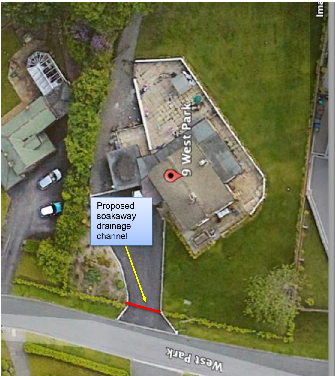
(Figure 5 – Position of proposed soakaway channel)
