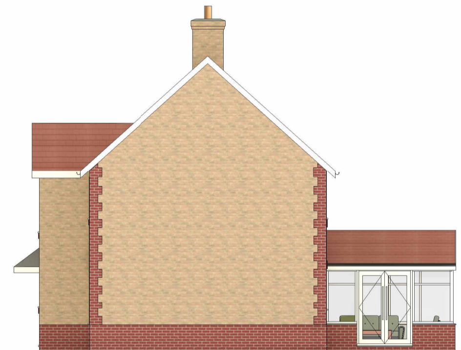
4 Proposed Side Elevation 1 1 : 100
