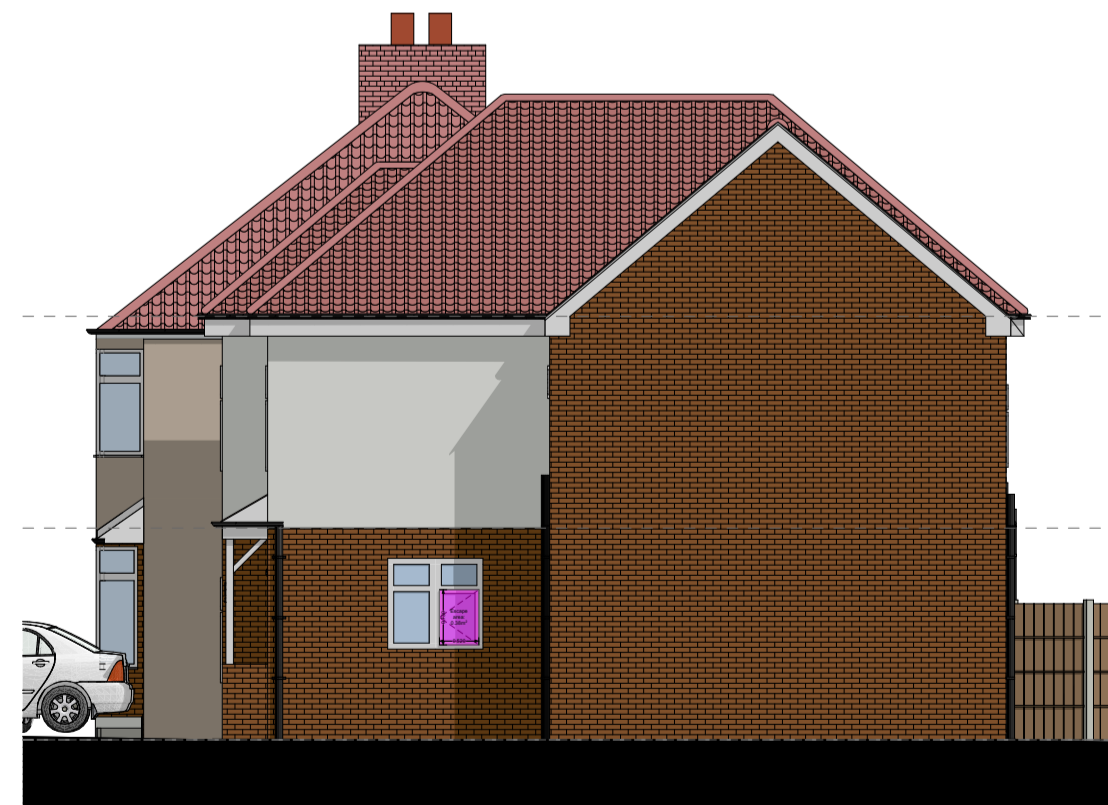
06 67A: West-facing flank elevation - emergency escape window 1:100
