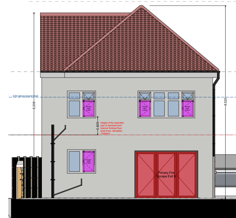
10 67A: Proposed rear elevation - emergency escape windows 1:100
