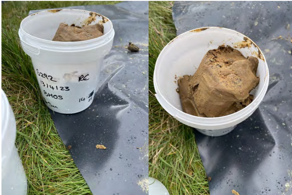
Photo 10—Example of disturbed samples taken
