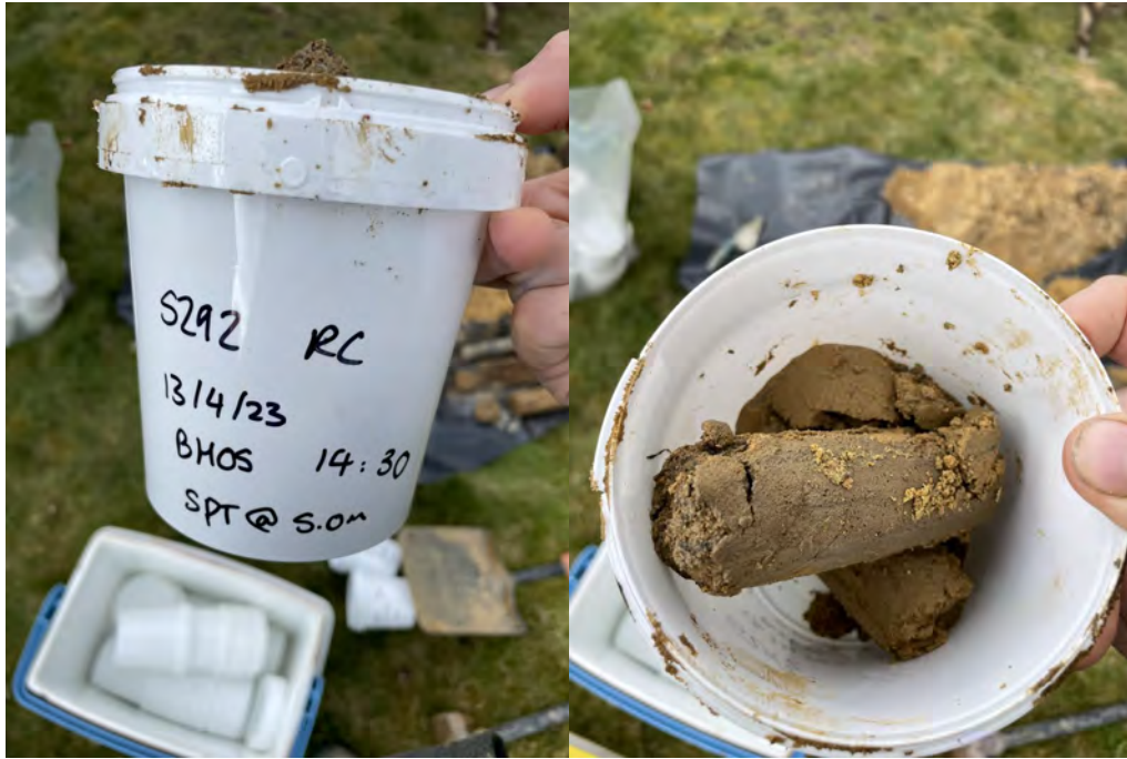
Photo 9—Example of SPT arisings
