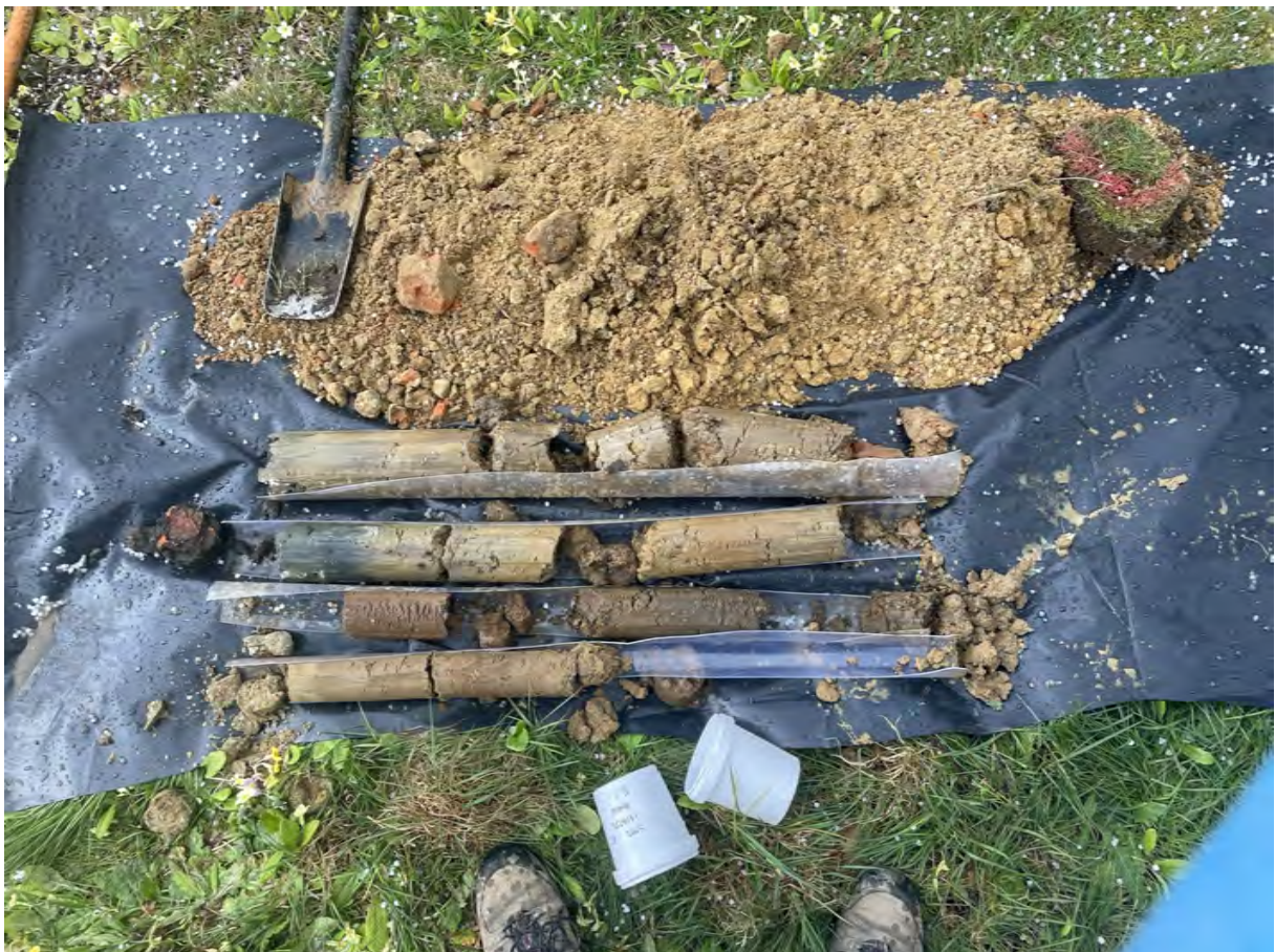
Photo 6—Example hand dug safety starter pit arisings and cores obtained from drilling
