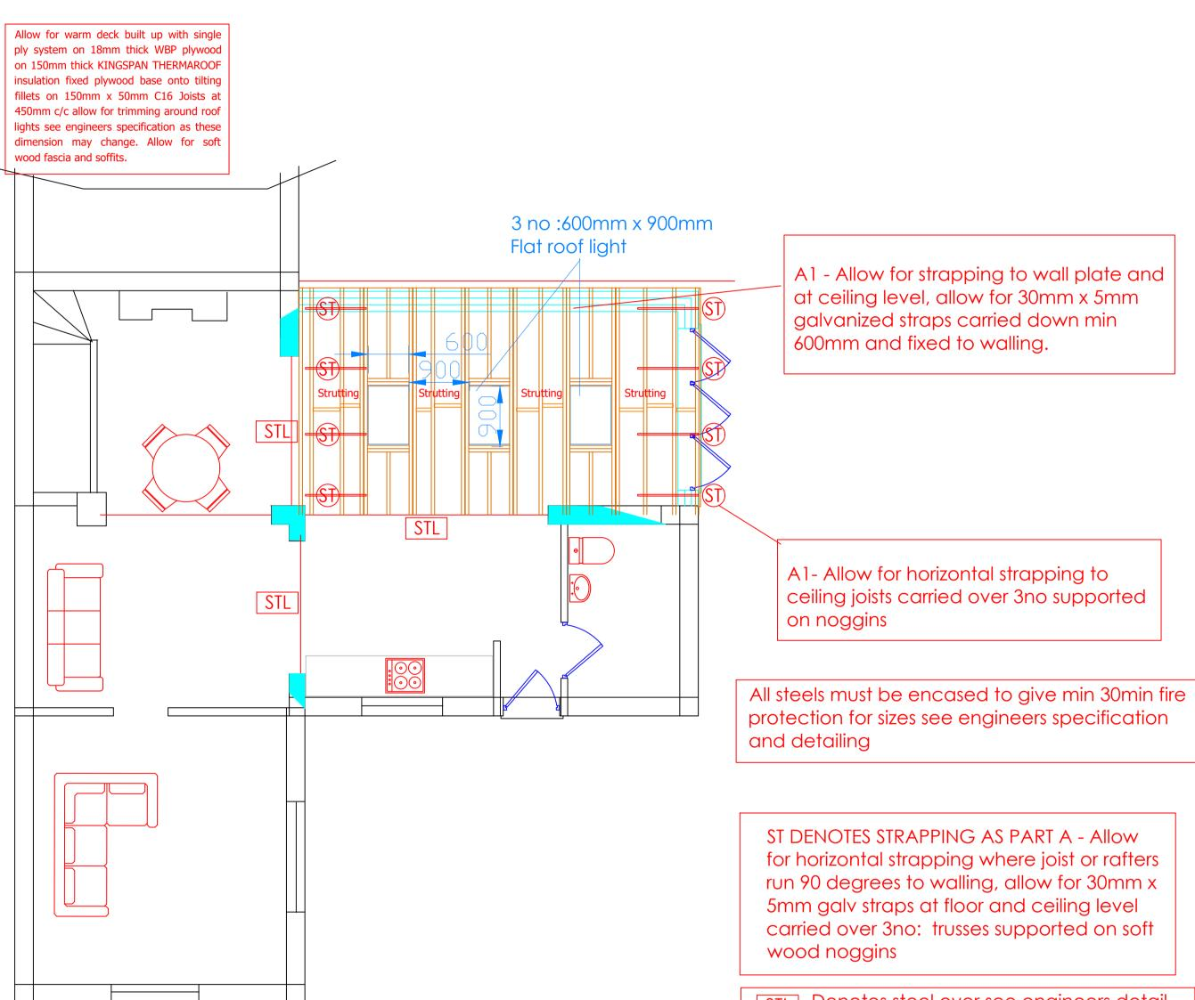
STL Denotes steel over see engineers detail and specification. All steel must be encased in plaster board to min 30mins protection
