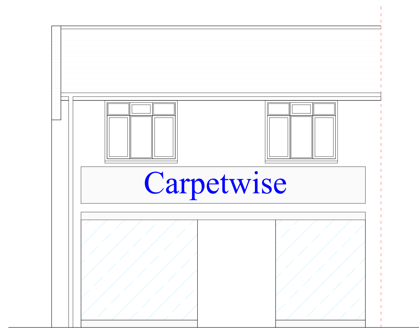
Existing Shop Front East Elevation Scale 1:50 @ A1
