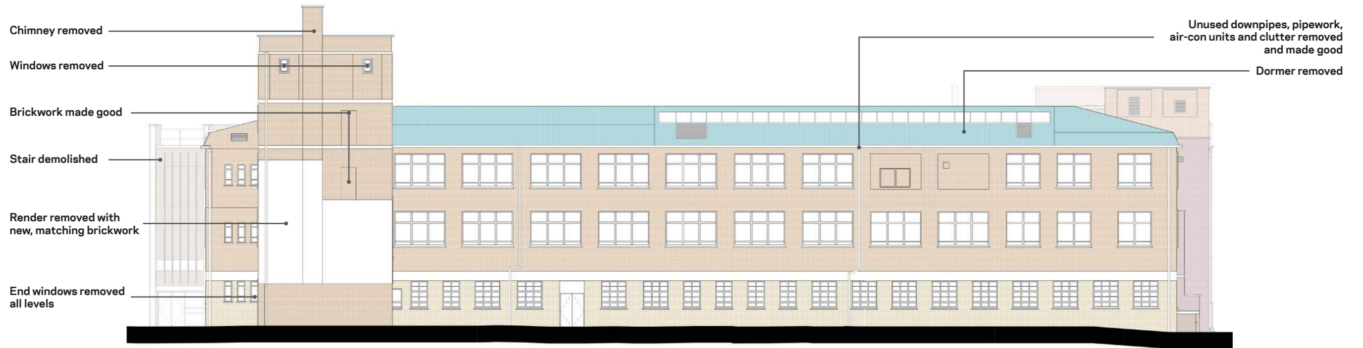
Existing north elevation
