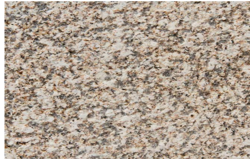
Granite kerbs and seating walls, flamed finish, or similar.
