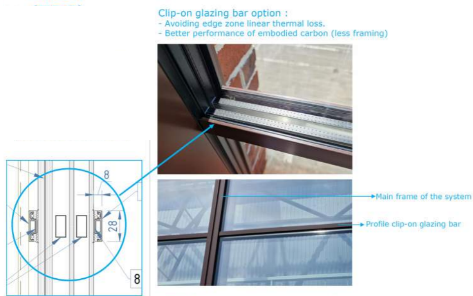
An alternative option of clip-on glazing bar for window mullion and transom.
