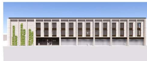
Study F • as D, but with opaque cladding retained on exposed side. • test of recessed wall hosting plants/creepers, and stone to top spandrel
