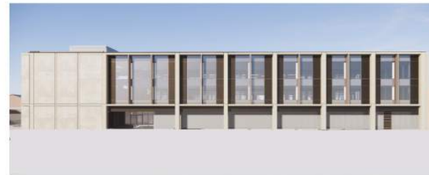
Study D • ground floor intermediate posts omitted to form wider bays • opaque cladding portion mirrored within bays (compromises shading)
