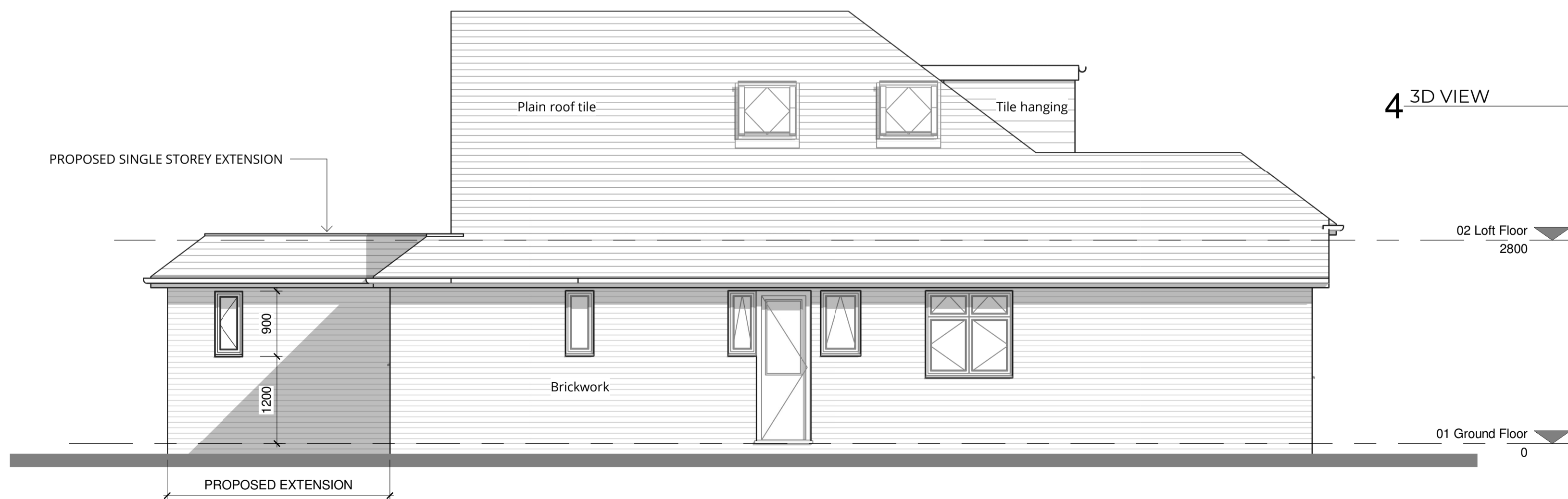
3 West Elevation DP 1:50
