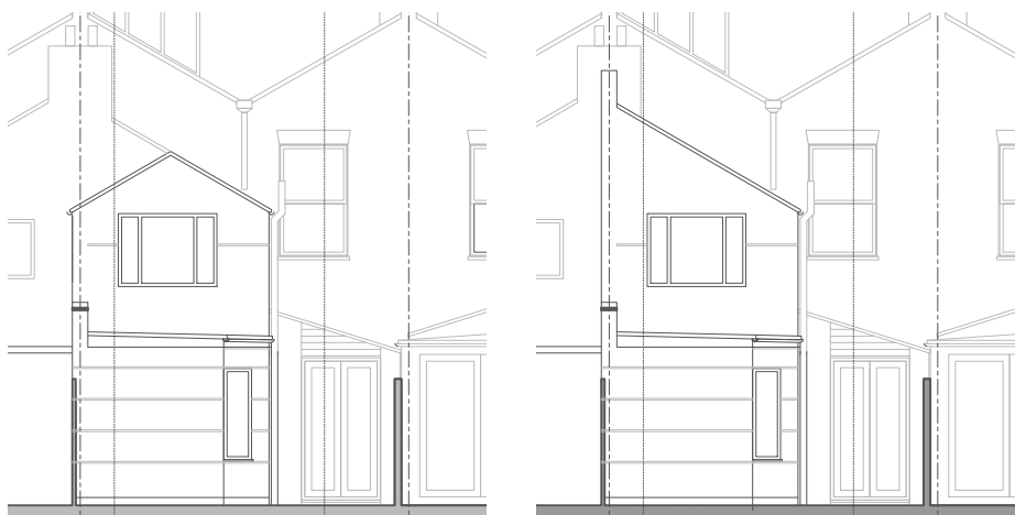
Fig. 10. Existing and Proposed sections illustrating relationship to the adjoining properties.
