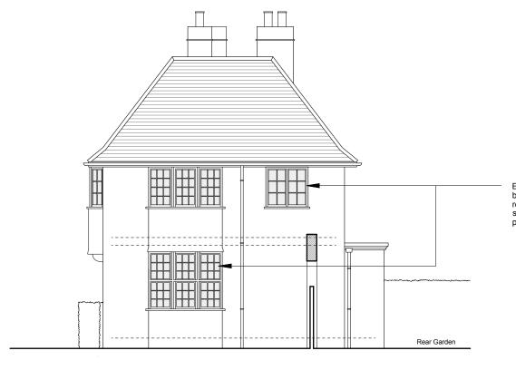
Existing timber windows to be carefully repaired and retained and fitted with slimline double glazed panes between glazing bars
