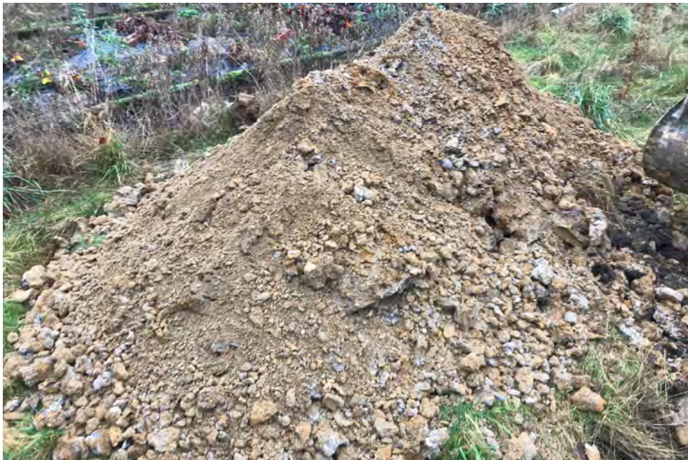
Soil arisings of trial pit SA3
