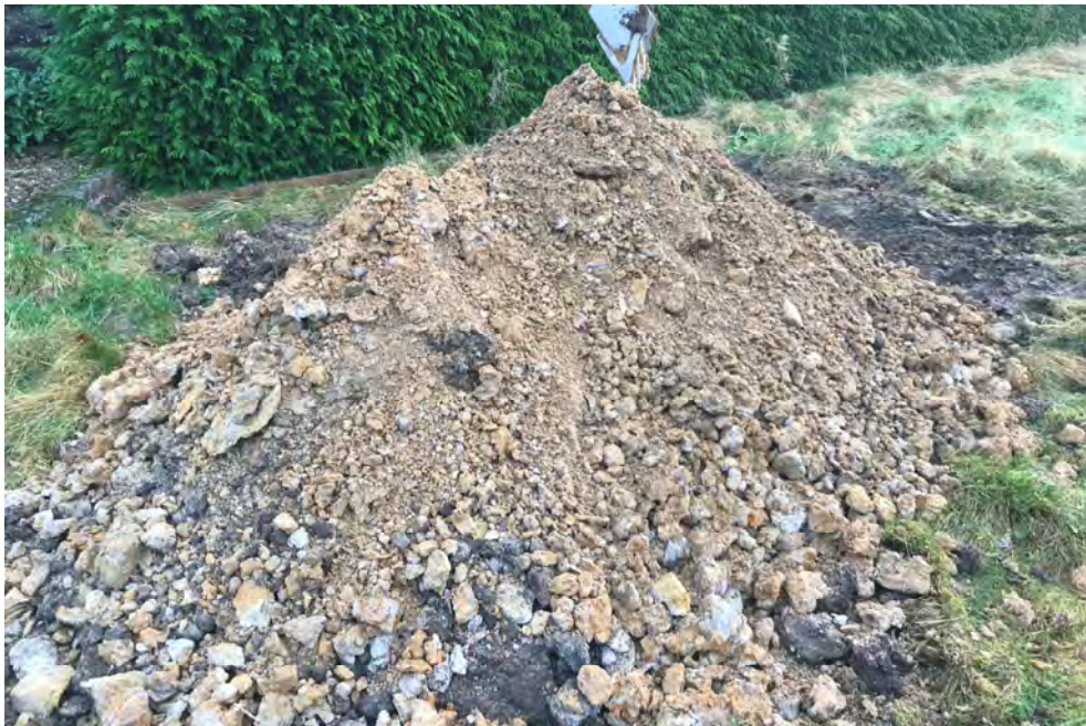
Soil arisings of trial pit SA2
