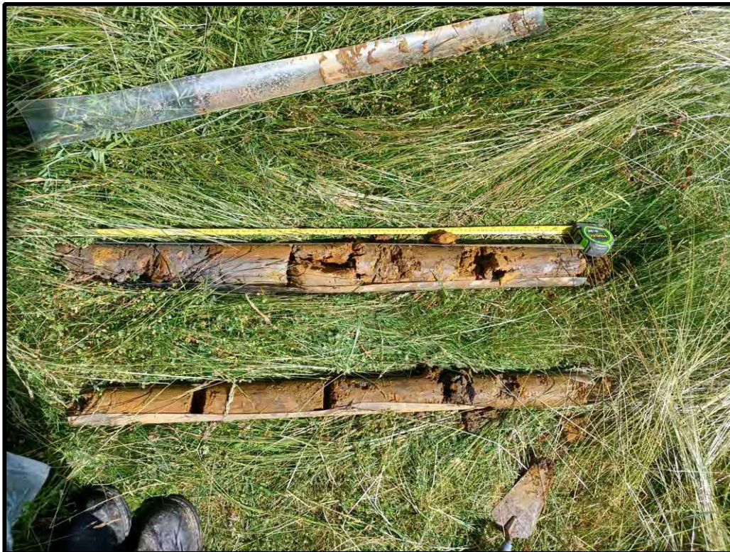
Borehole Core 1.0-3.0m
