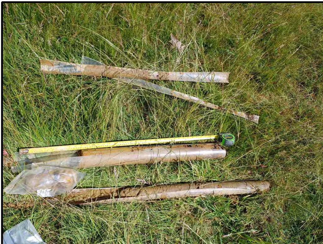
Borehole Core: 1.00-3.00m
