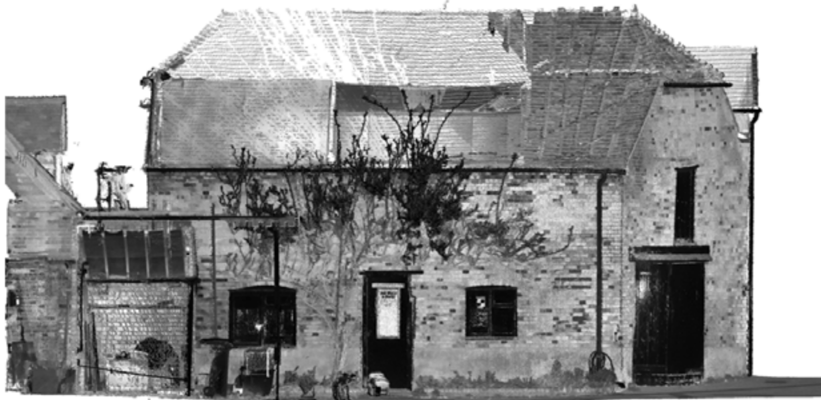
Point cloud survey: North elevation
