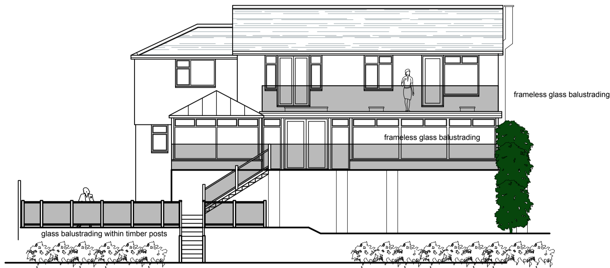
Existing Approved Rear Elevation
