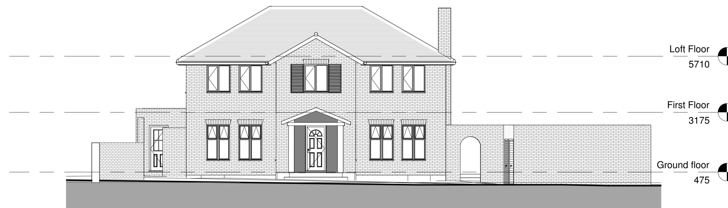
4 Existing West Elevation 1 : 100
