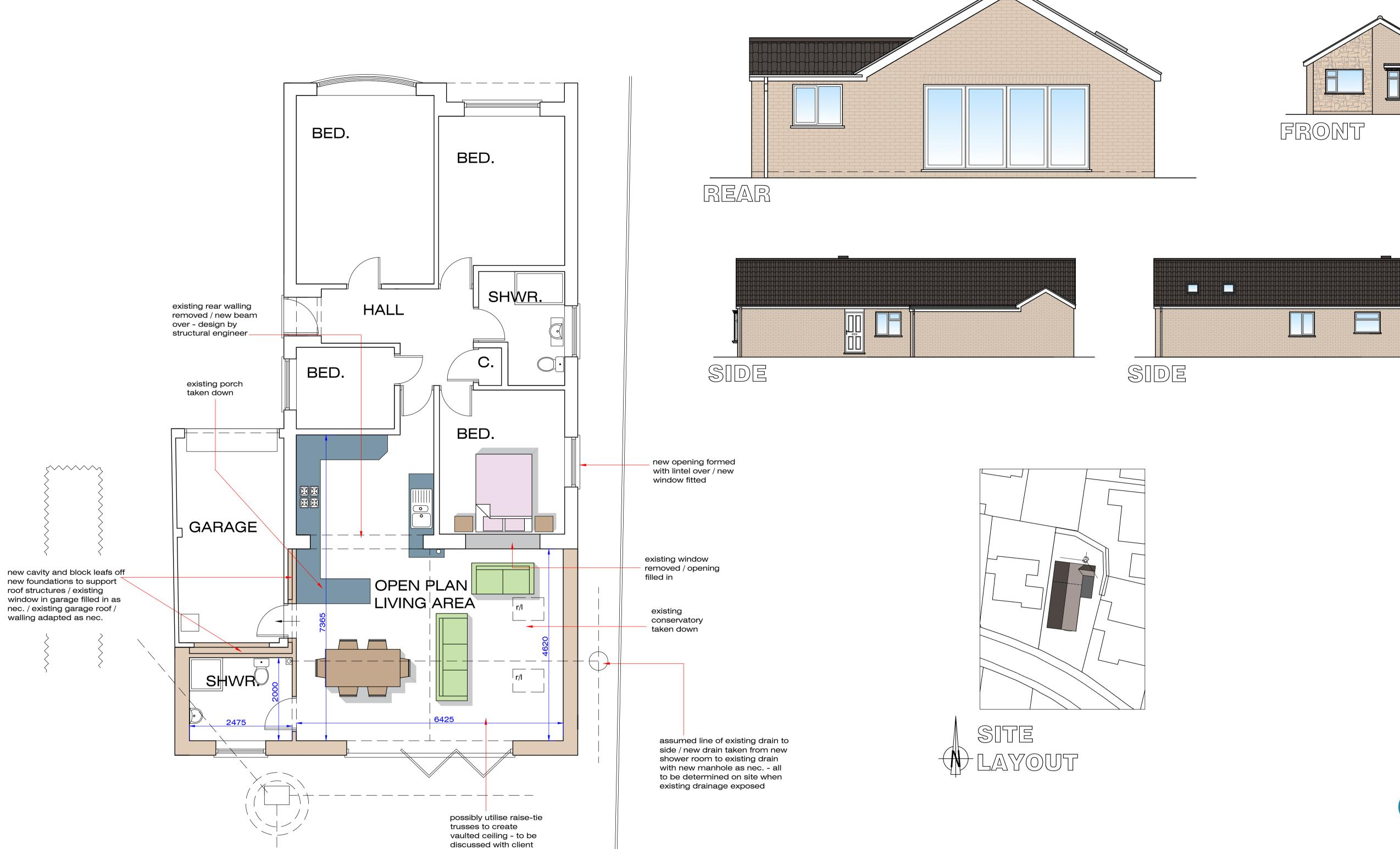
FLOOR PLAN # due to proximity of extension to Anglian Water drainage, and depth of drainage, piles and ring beam are to be designed to ensure no loadings are placed on existing drainage / beam & block floor to be formed with spine wall under open plan living area - design of foundations by structural engineer / exact drainage layout to be determined on site prior to work starting due to limited access at time of survey #
