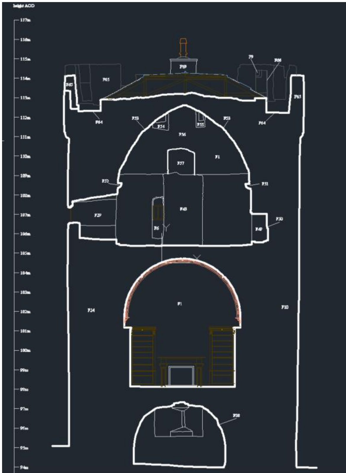
Fig. 3 CAD cross section showing the construction of the Drum Tower, with the Library inserted into the first floor in the 19 th century, copyright NTS
