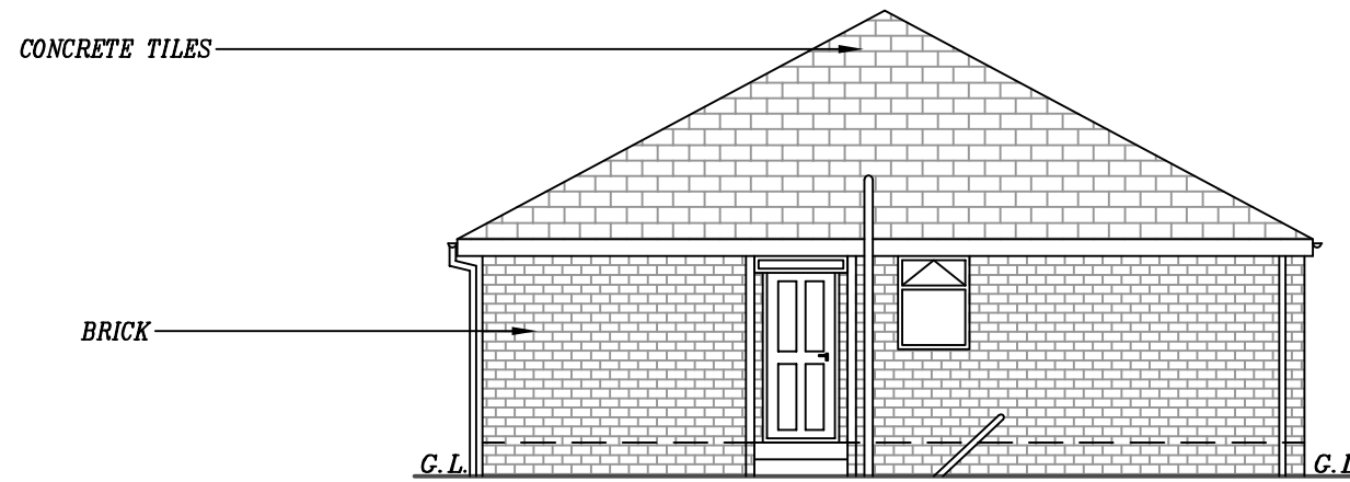
EXISTING SIDE ELEVATION
