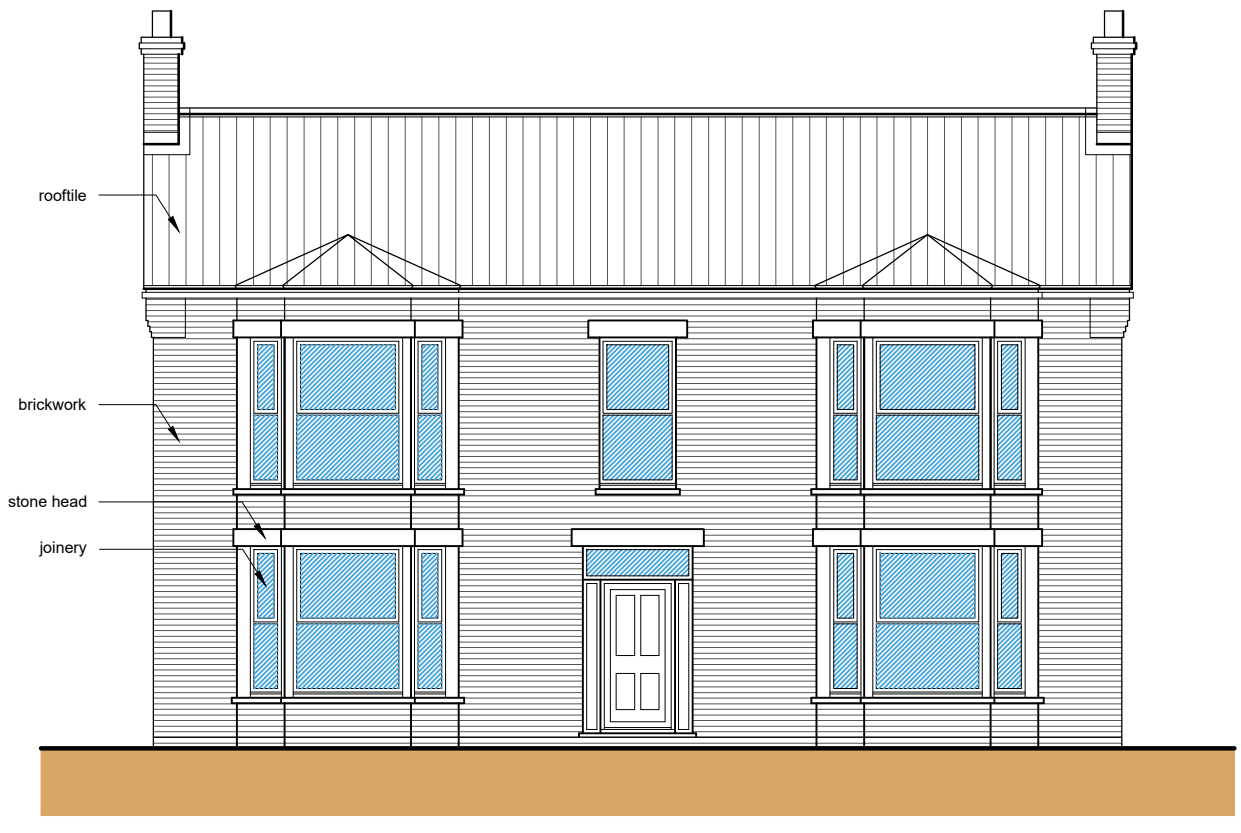
Front Elevation (NW) Scale 1:100 metres
