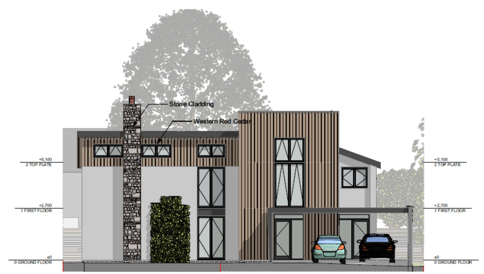
Plot 1 East Elevation 1:100
