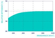
Typical module performance under low irradiance conditions in comparison to STC conditions ( $25 \,^\circ$ C,  $1000 \,$ W/m<sup>2</sup>).
