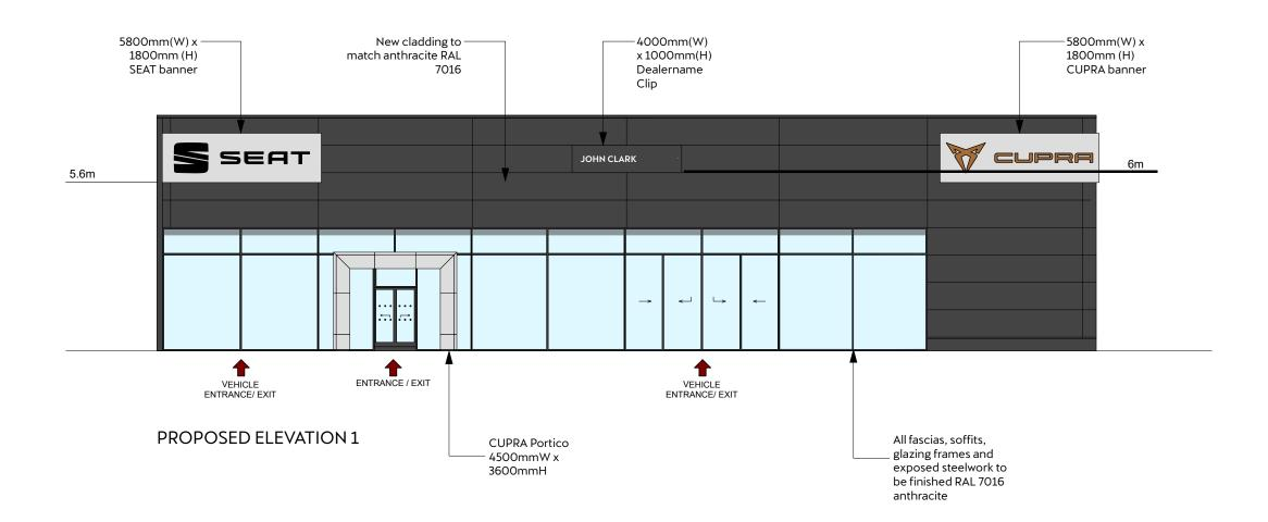
Seat fascia sign - static and internal illumination by white LED's ACM, aluminium and acrylic in grey and black. Fitted to the building by Tek screws
