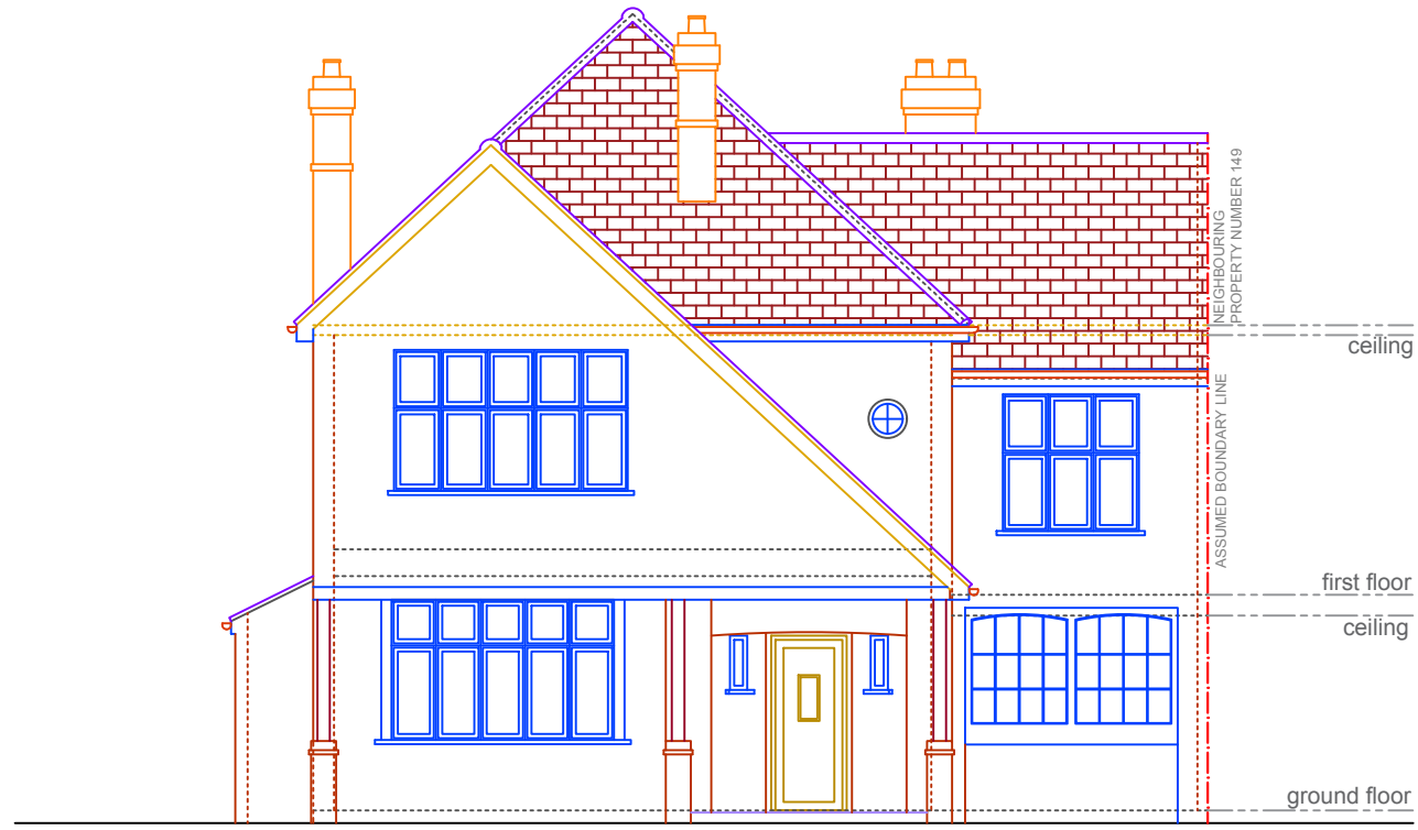
7 FRONT ELEVATION- EXISTING (NO CHANGES PROPOSED) 1:100
