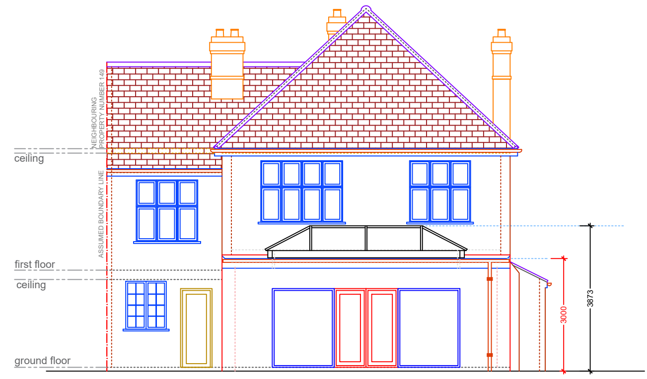
9 REAR ELEVATION - PROPOSED 1:100
