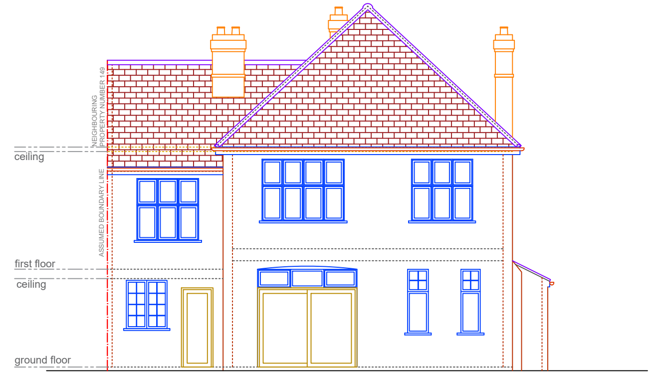
8 REAR ELEVATION - EXISTING 1:100
