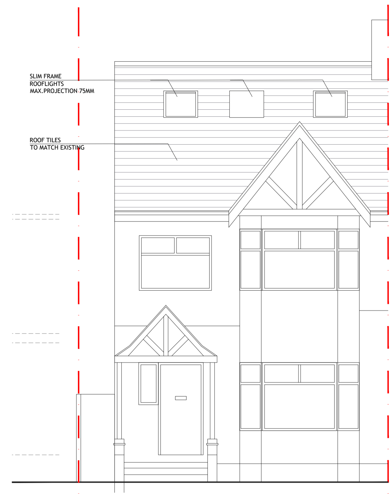
PROPOSED FRONT ELEVATION SCALE 1:50 @ A1 & 1:100 @ A3
