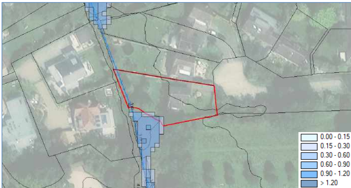
Figure 9 EA Long Term Flood Risk Maps (Depths) – High Risk of surface water flooding (source: EA Long Term Flood Risk Maps), site bordered red.
