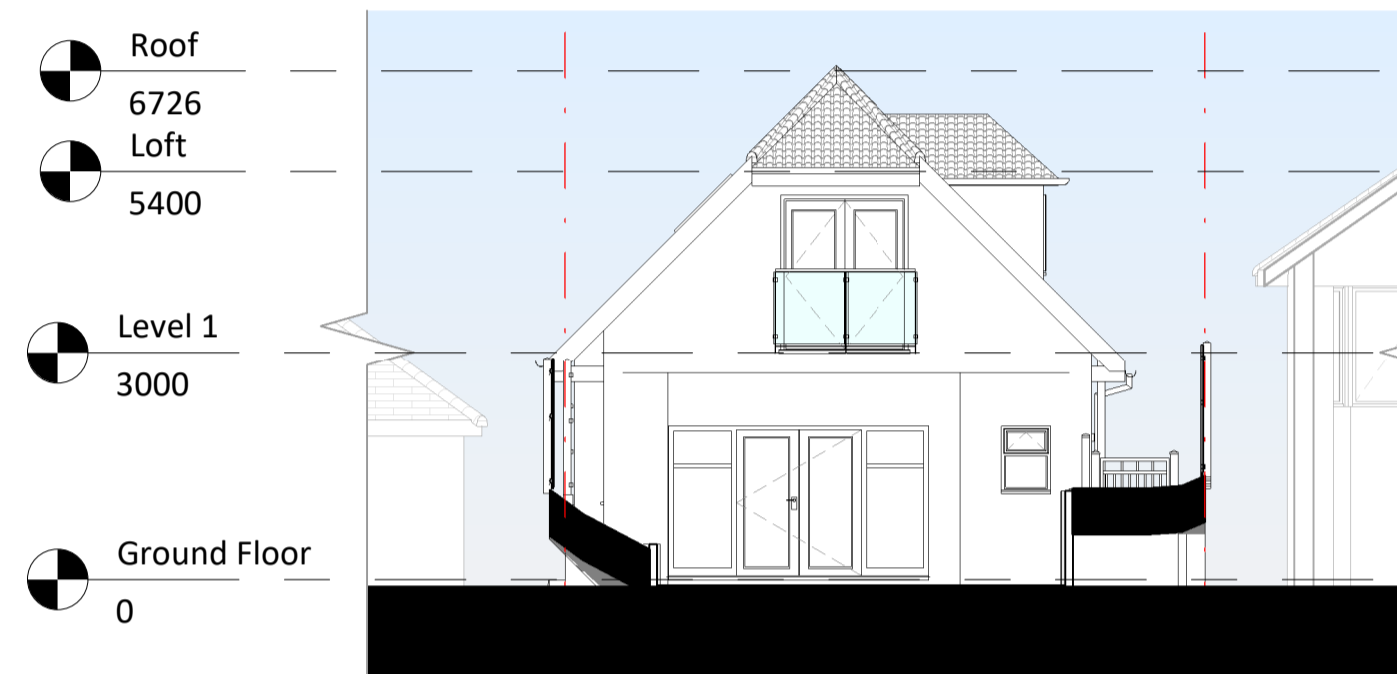
7 Existing Rear Elevation 1 : 100
