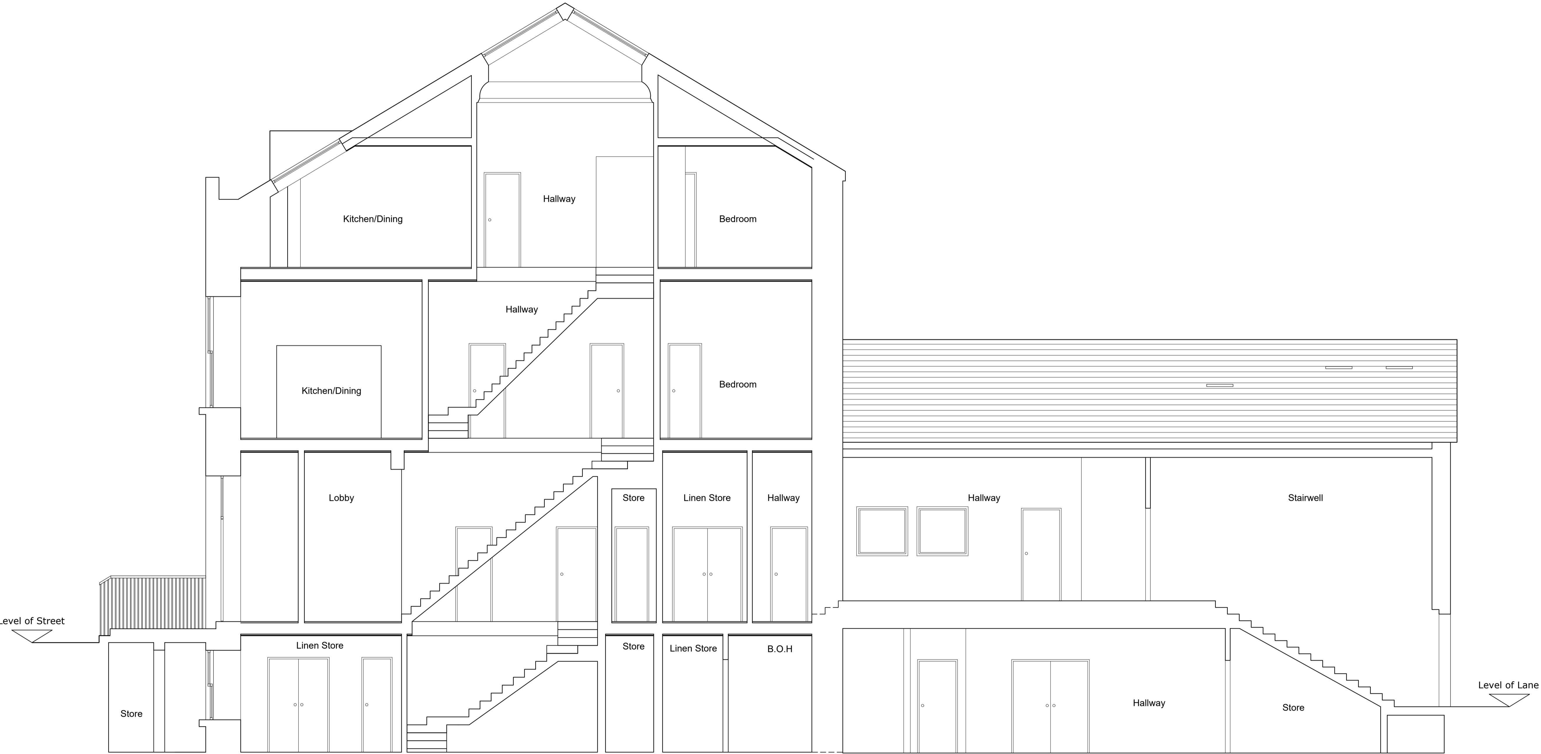
Section B-B as Proposed, 1:50
