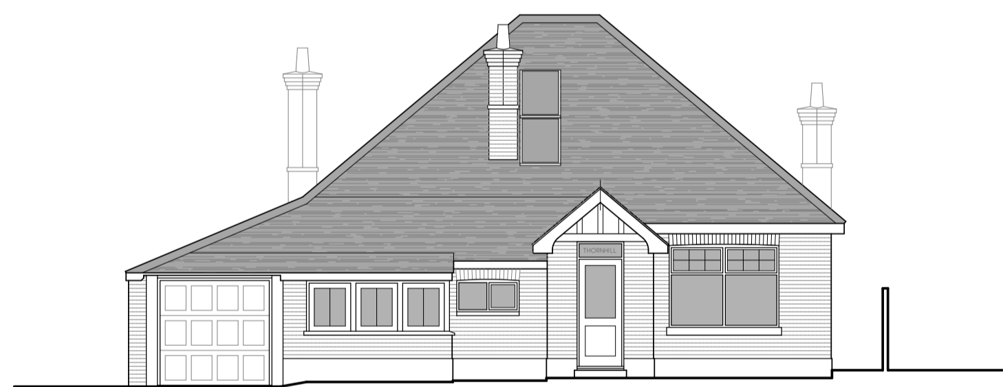
FRONT ELEVATION 1:100 WEST
