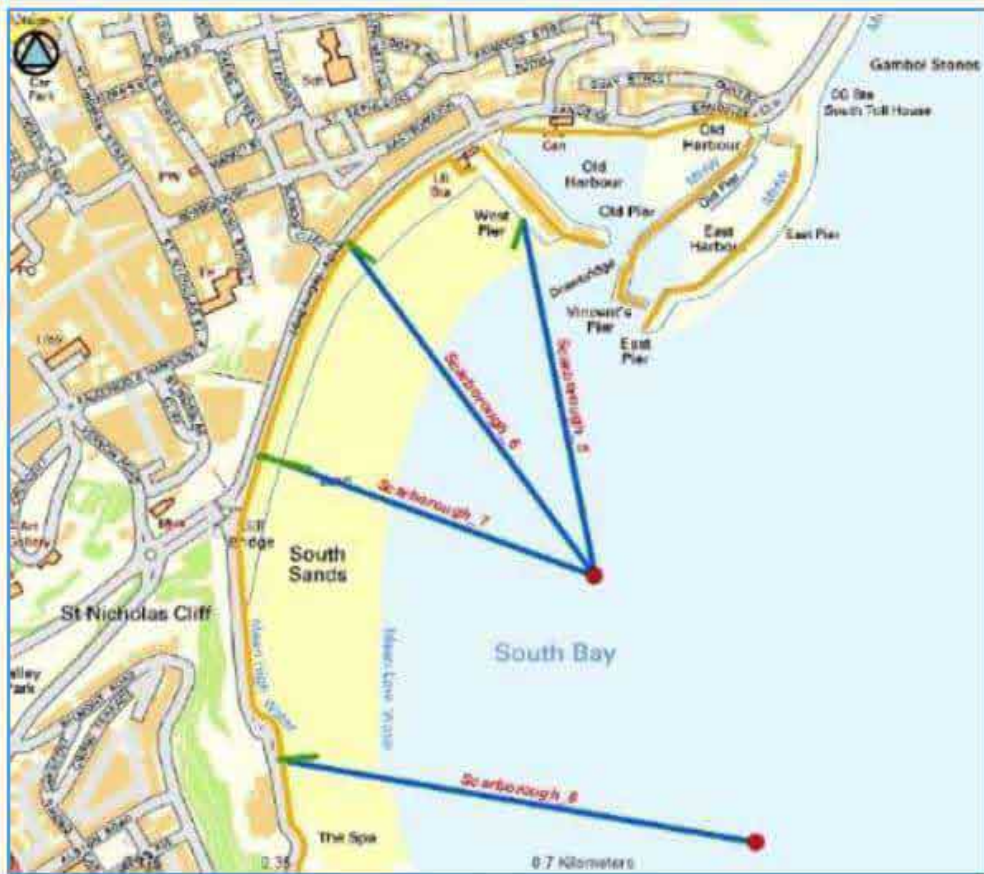
Figure 1-8: SWAN 1D transects simulated as part of the Yorkshire Flood Forecasting Update 2017
