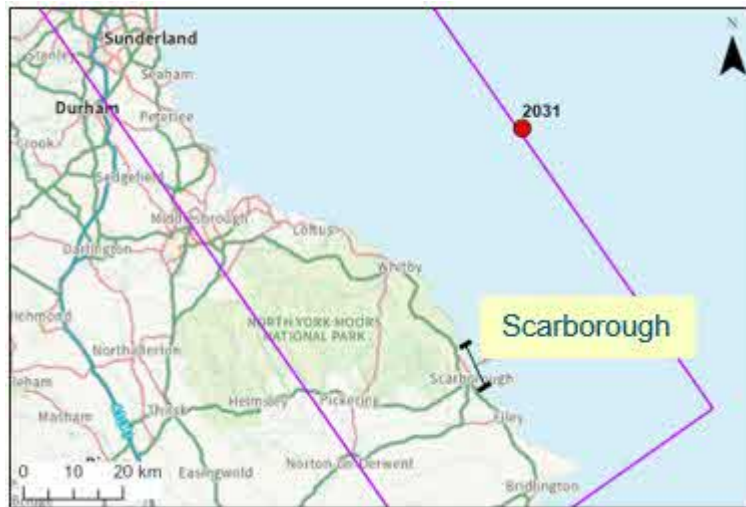
Figure 2-1: UK Met Office wave hindcast point P2031 (red point) in relation to Scarborough and SoN SWAN model (purple line)
