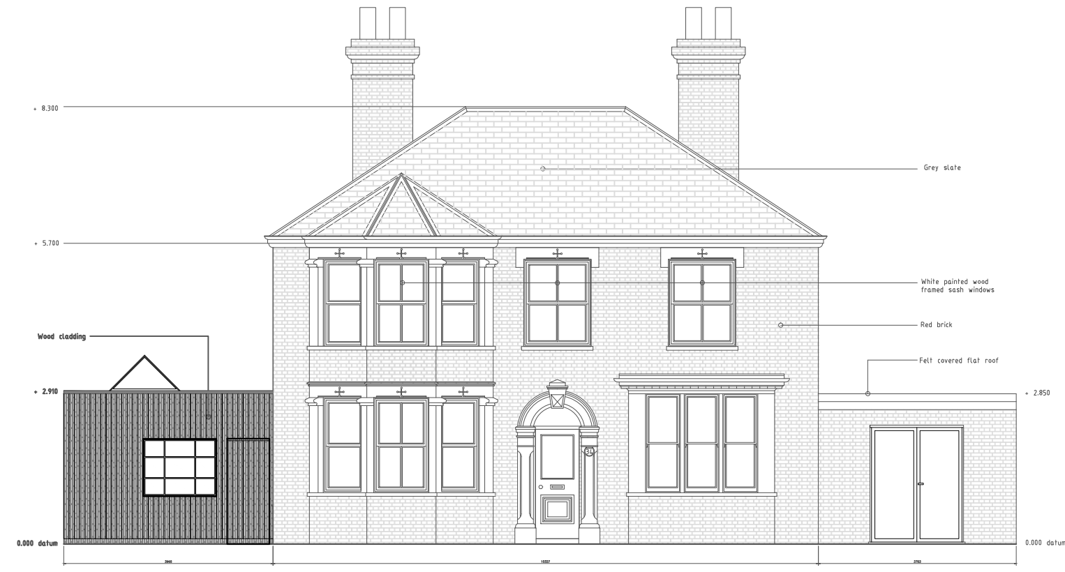
Front Elevation (South facing)
