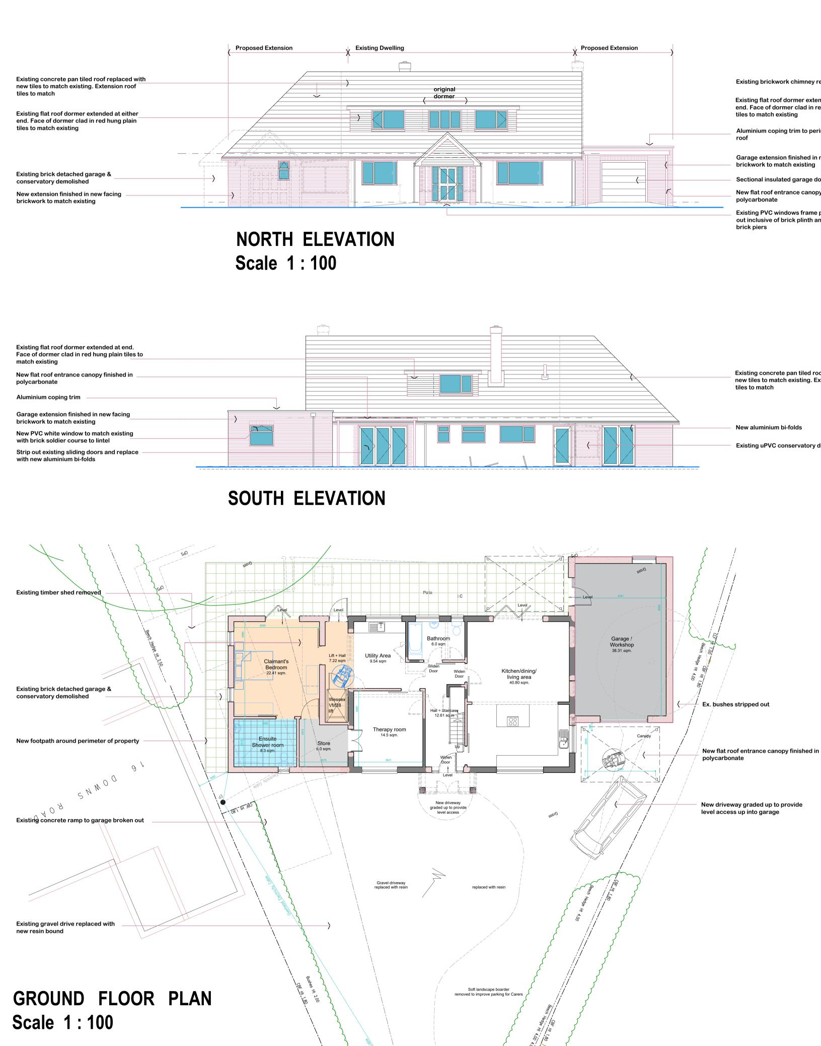
Existing brickwork chimney removed. Existing flat roof dormer extended at either end. Face of dormer clad in red hung plain tiles to match existing
