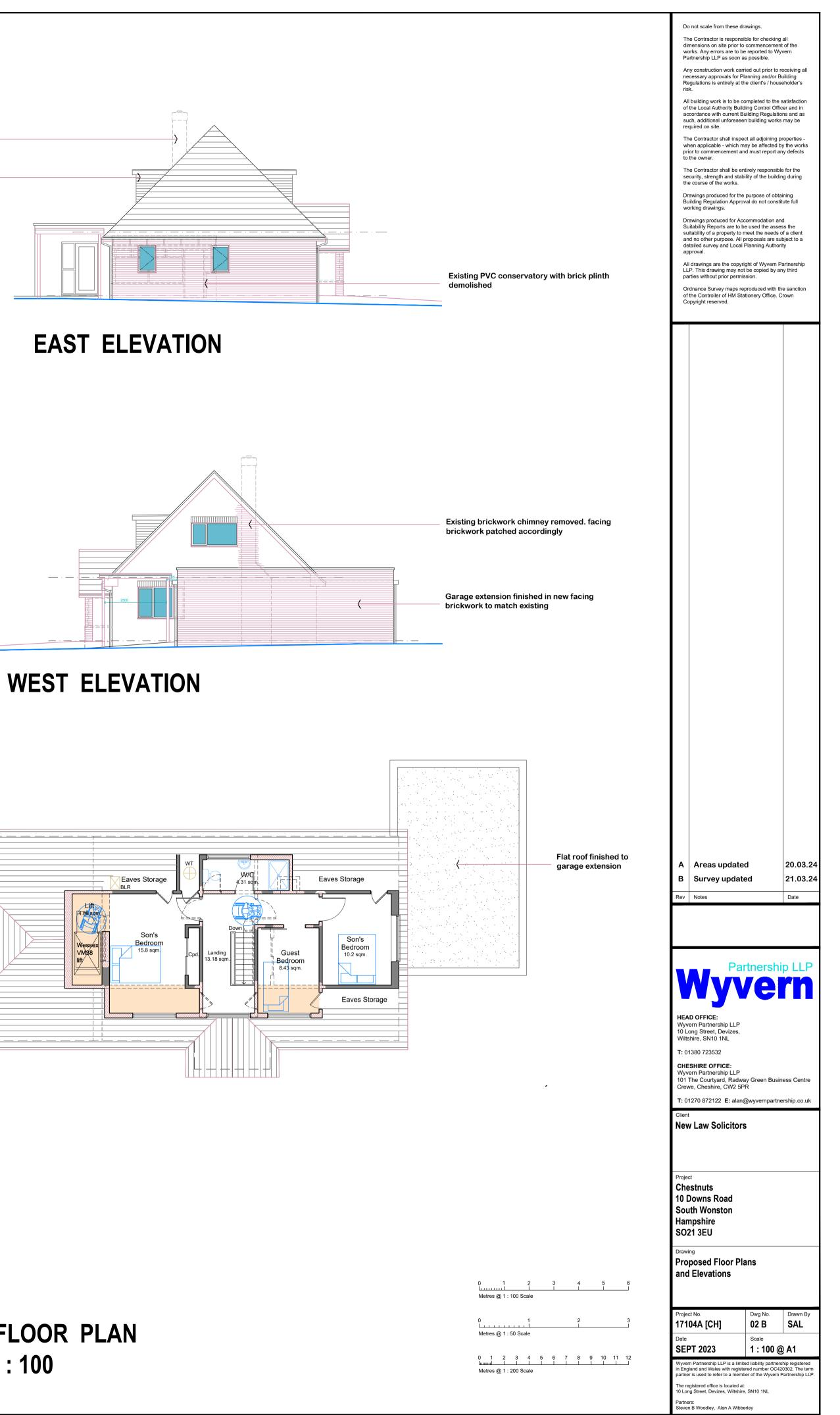
Existing concrete pan tiled roof replaced with new tiles to match existing. Extension roof
