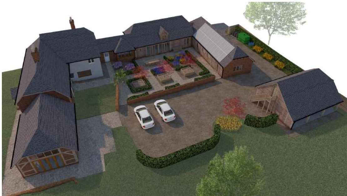
Figure 43; Aerial rendered view showing the site from the East. This shows the relative positions of the ground floor extension to the right of the cart shed, and the garage and store building. The sense of the courtyard garden and revised parking area is also shown.
