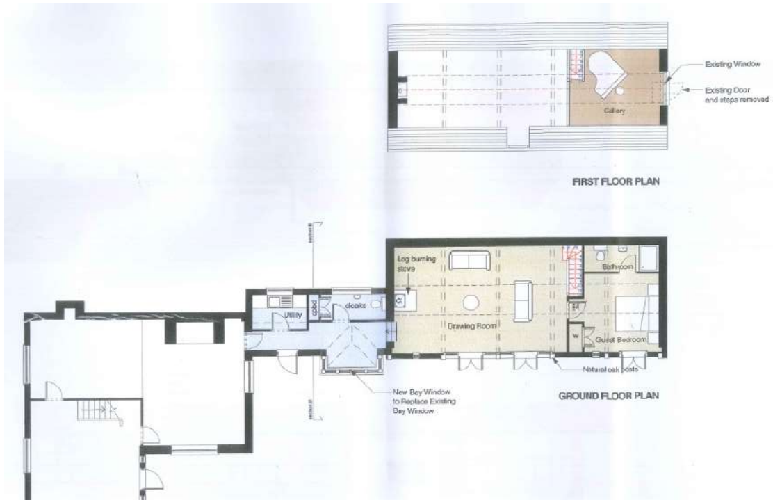
Figure 27; Reduced plans illustrating the works consented under 21921/009 and 21921/010 for the conversion of the former cart shed.
